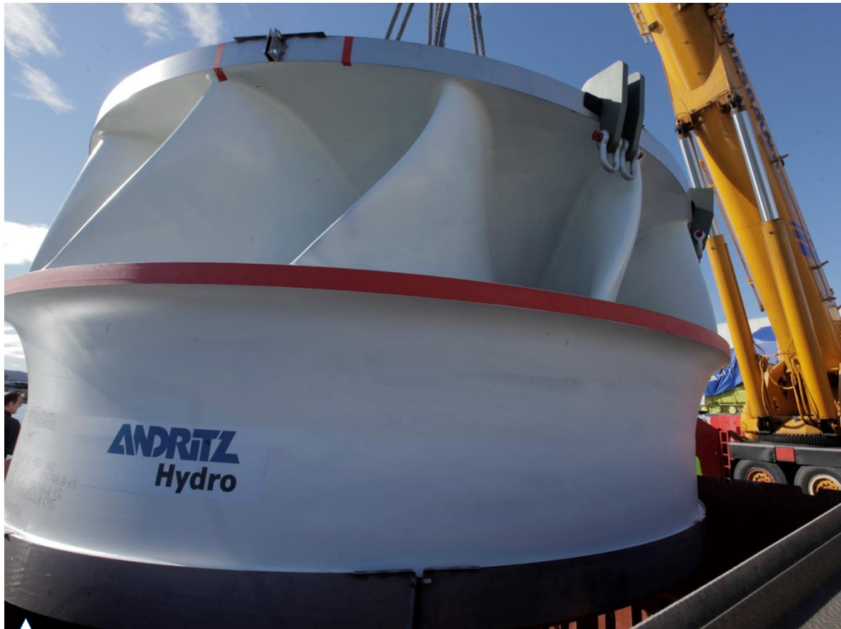
ANDRITZ supplies two Francis turbines for the Mica hydropower plant in British Columbia, Canada. Each turbine has an output of 520 megawatts and a runner diameter of 5.6 meters
